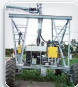
Hose Drag Buried Wire Guidance New Zealand
