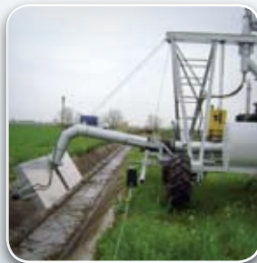
Side Ditch Feed Above Cable Guidance Ukraine
