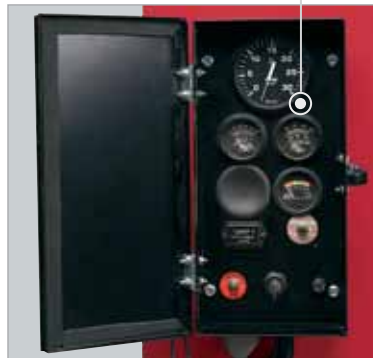
Standard rodent-proof instrument panel.
