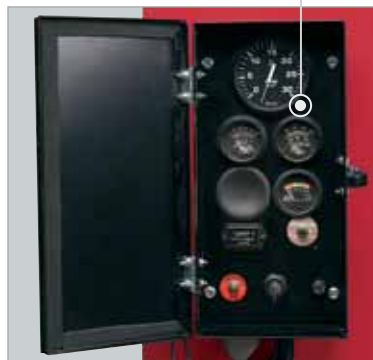
Standard rodent-proof instrument panel.
